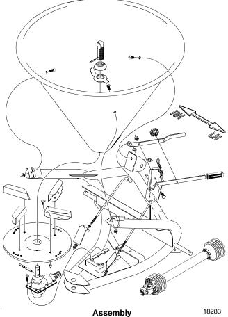
Assembly Figure 1-1 **Optional Equipment Assemblies**
